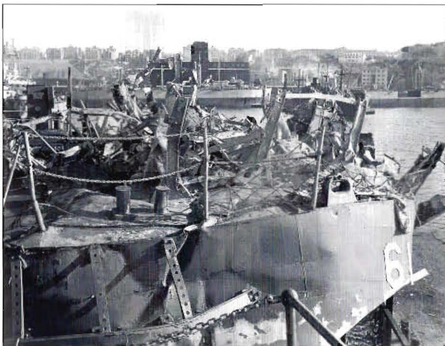
Upper right: USS Murphy (DD-603) was sliced in half by the tanker Bulkoil . The forward portion of the ship sank within minutes. The after portion is seen here at New York Navy Yard on 23 October 1943, two days after the collision.
