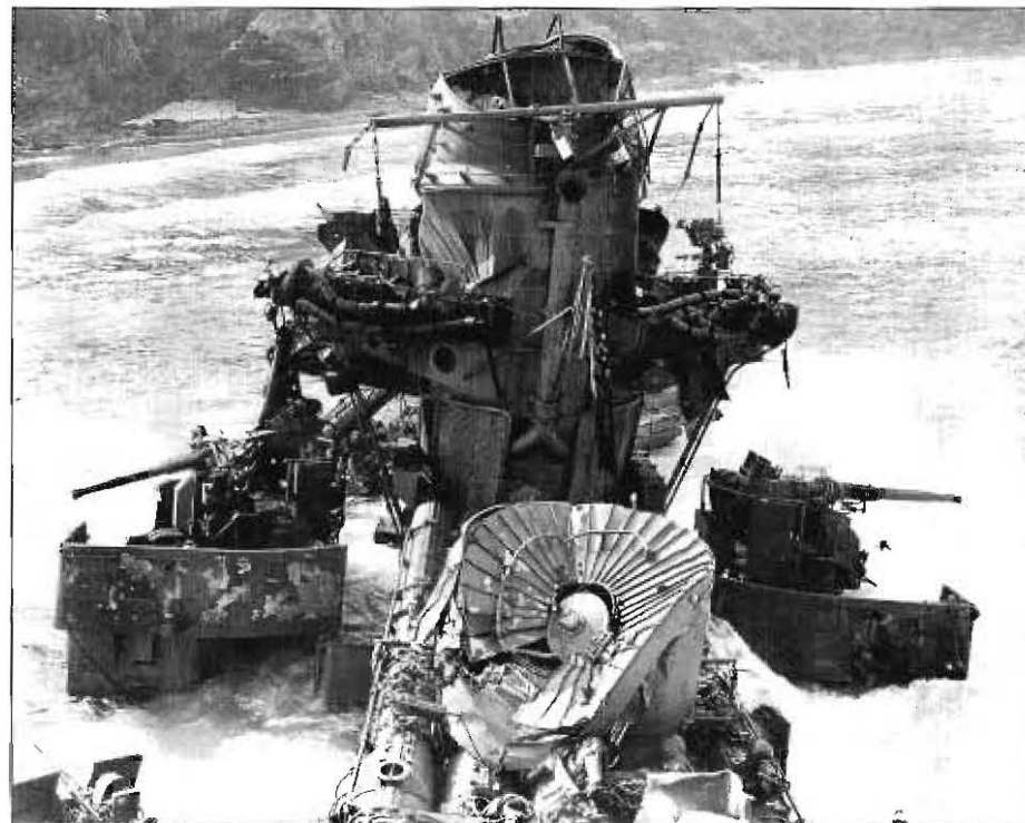
Above: USS Halligan (DD-584) struck a mine on 28 March 1945. The explosion detonated her forward 5" magazines. The ship forward of the forward stack was destroyed.
